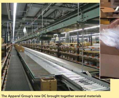
The Apparel Group's new DC brought together several materials handling automation technologies, including roller and spiral conveyor, tilt tray sortation, pick-to-light and RF picking technologies and a garment-on-hanger rail system.
